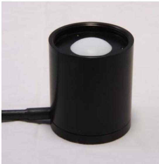
The PMA 2132 Quantum light detector(PAR)measures the photon flux in wavelength range from 400 to 700 nm.
