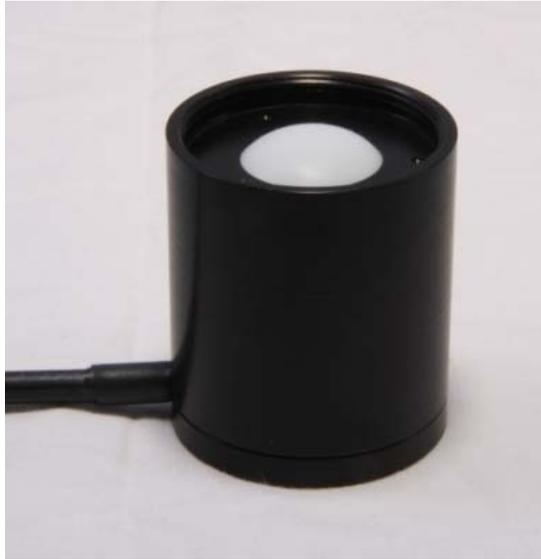
The PMA 2121 blue light safety sensor offers an accurate, easy, inexpensive way to measure the blue light radiation hazard to eyes for a wide range of occupations. Such exposure, according to numerous medical studies, can inflict permanent and irreversible damage to the eye causing visual field defects and visual impairment.
