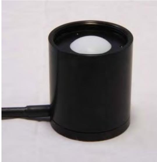
The UVB sensor PMA 2101 biologically-weighted erythema gives an accurate measurement of ultraviolet radiation from sunlight or artificial light sources, also called sunburning UV radiation (SUV). Its spectral response follows closely the erythema action spectrum. The detector has angular response very close to an ideal cosine function (Lambertian response) making it suitable for measurements of diffuse radiation or radiation generated by extended sources.
